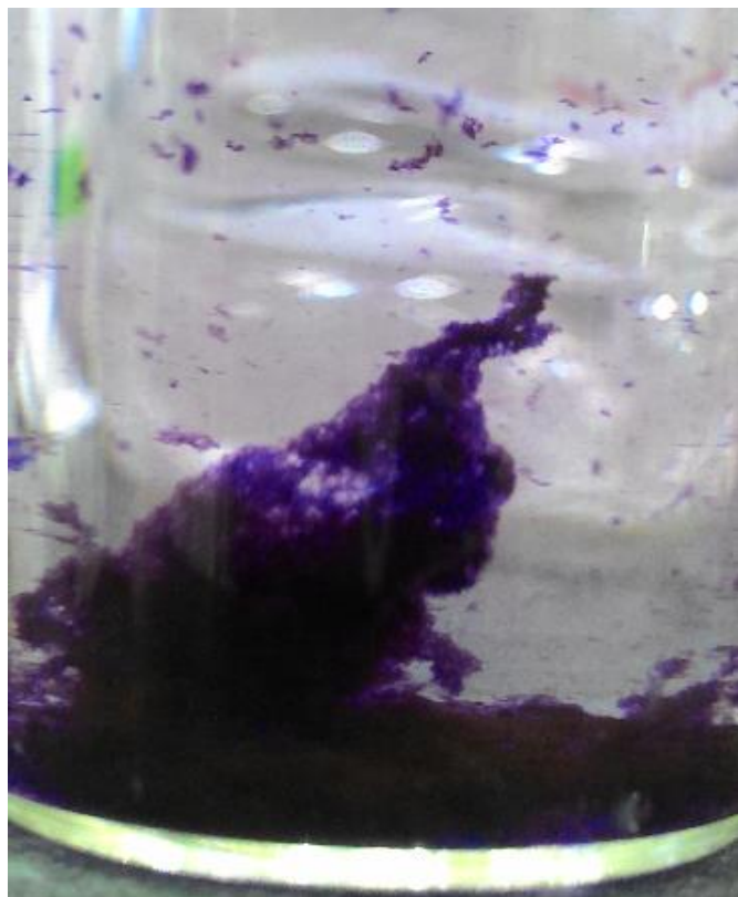
Figure 3. The aggregated mesh-like DB71 using undiluted seawater that settle at the bottom of glass vial before filtering with distilled water.
