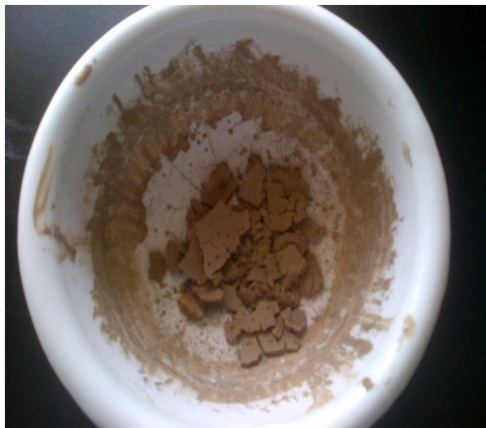
Figure 3. Representation of the extracted alginate from pulverized seaweeds of light brown colouration.
