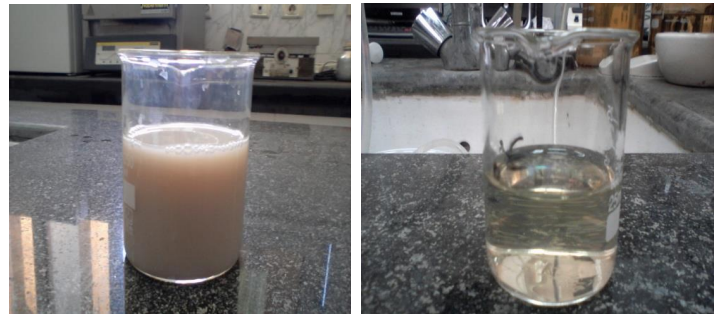
Figure 10. Images of industrial wastewater from El-Sewedy cables industries (a) before adsorption and (b) after adsorption of copper ions.
